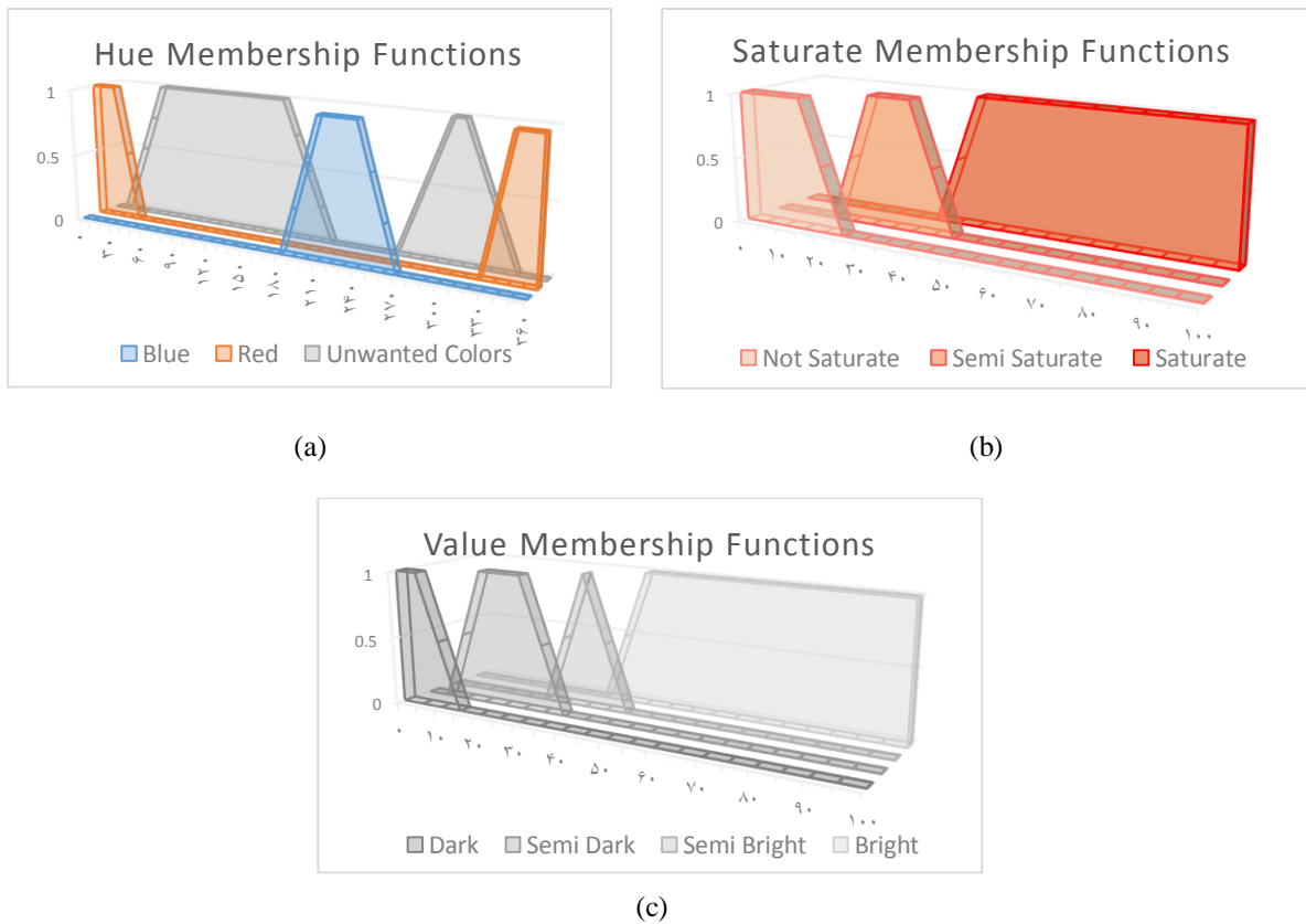
Fig9. Membership Functions of Fuzzy Inference System for Create Fuzzy Image, (a) Hue Membership Functions, (b) Saturate Membership Functions, (c) Value Membership Functions.
